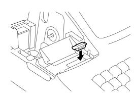
Insert the new Ink Roller in the slot of the carriage by pushing it all the way in until it is firmly settled with a "click" sound.
